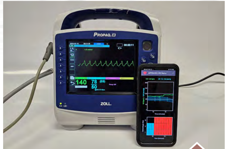
The APPRAISE-HRI consists of a commercial vital-sign monitor and an AI app running on an Android smartphone.
