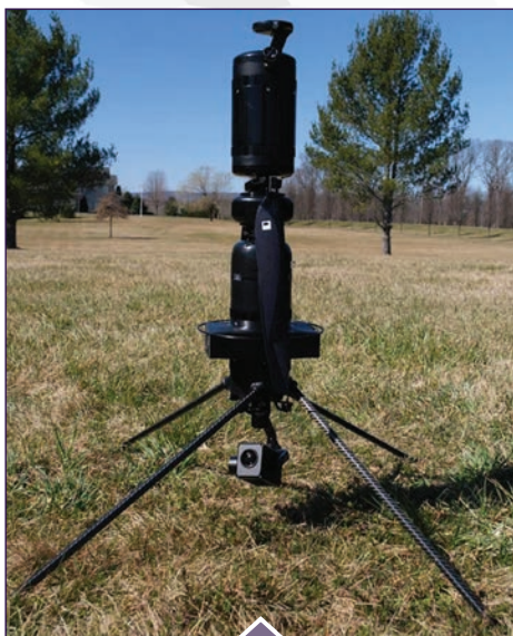
The VISTA technology (payload) integrated into the Ascent AeroSystems Spirit UAS.
