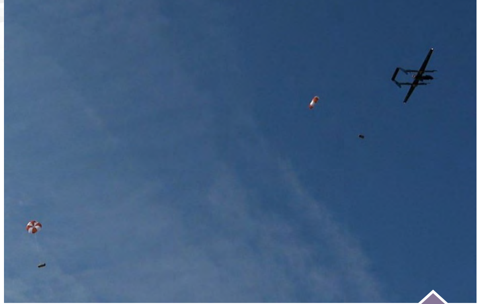
Crimson system delivering medical supplies via parachute drop to satisfy a field user request.
