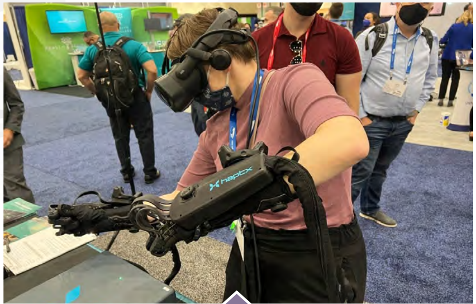
Chrissie Phillips using haptic feedback gloves. Although these are designed for creating real haptic feedback in a VR environment, they can be modified through their APK to track finger and hand movements in a real world scenario.
