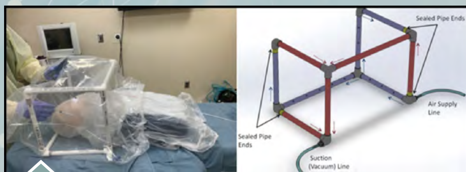
Figure 1: Original CAMIC Design - From EUA Documentation showing CAMIC prototype (left) and CAMIC Design Schematic (Right)
