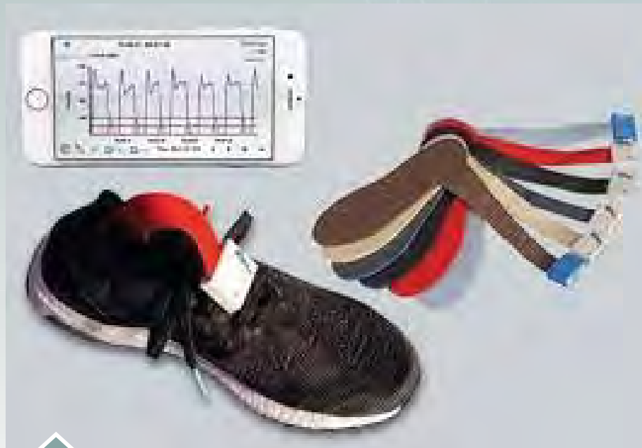
Figure 2: Loadsol® Insole with iPhone and Shoe
