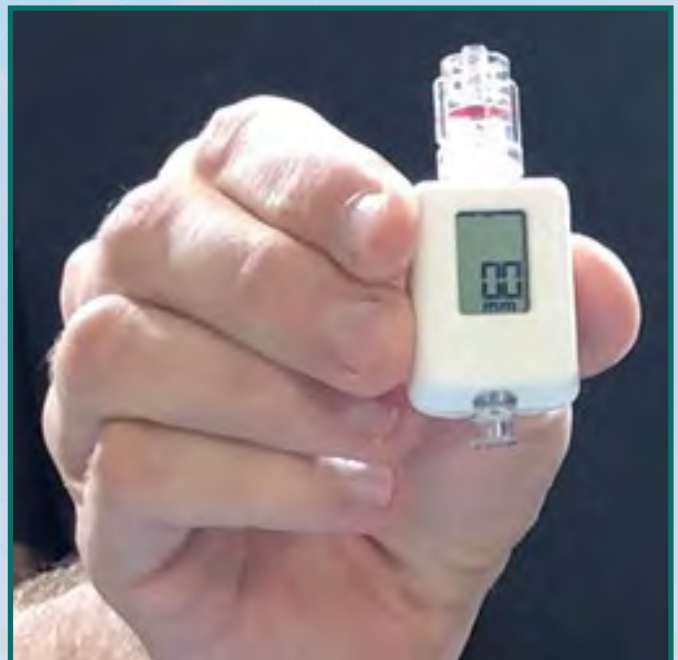
Figure 1. The COMPASS® device from Centurion Medical Products. Compact, disposable, battery powered mean arterial pressure monitor.
