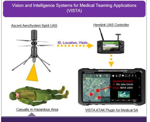
Diagram of VISTA, a computer vision software capable of stand-off casualty identification and physiological vitals signs assessment deployed on a standard Uncrewed Aerial System (UAS).
