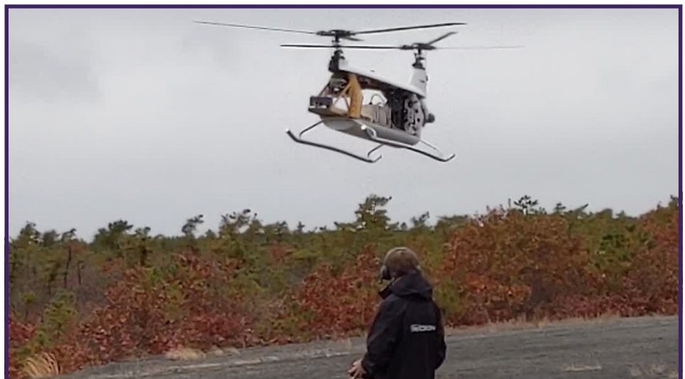
DP-14's “maiden-flight” event performed without the exterior skins of the aircraft to prove out mechanical performance and system stability during a manually controlled flight.
