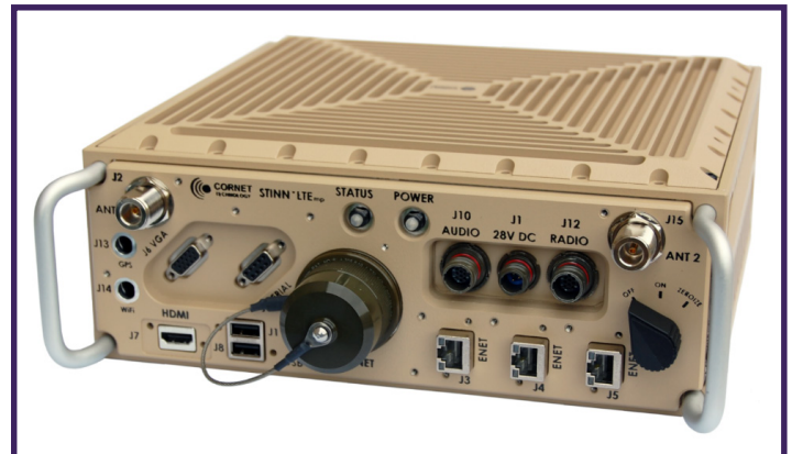
CORNET Technology's STINN LTemp Manpack 4g LTE Deployable Base Station (Cell Tower in a Rucksack)
