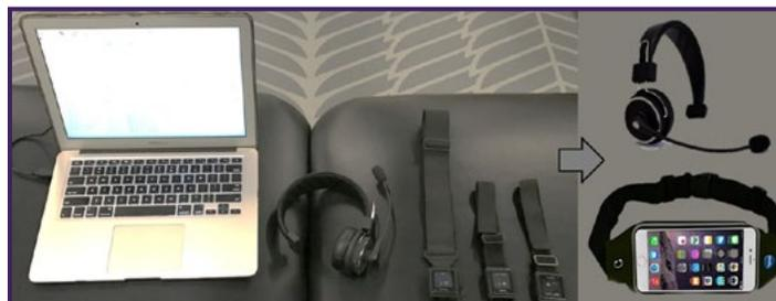
**Figure 1: The assessment tool consists of a wearable IMU system, wireless headset and automated Dual-Task protocol. The desired end state is to package the assessment into universally available smart phone based application.**
